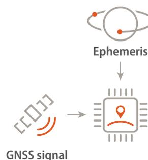
Figure 10: Snapshot-based position determination on the device
