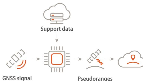
Figure 9: transmission of pseudoranges based on a snapshot of the signals
