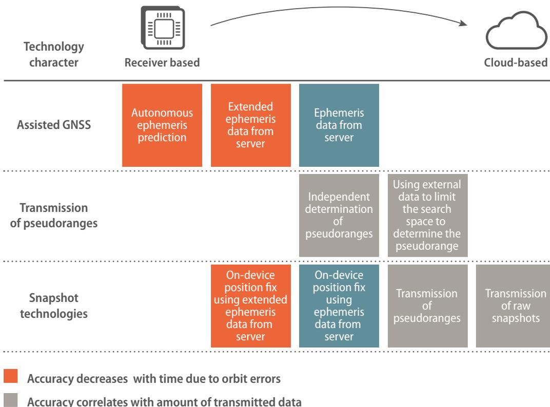
Figure 3: From receiver to cloud: GNSS optimisation techniques
