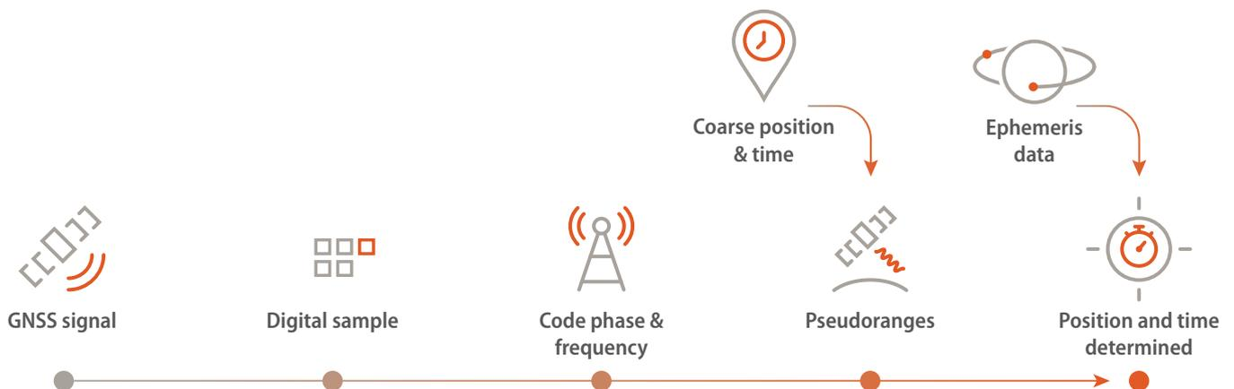
Figure 7: Snapshot positioning
