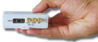
« GNSS Handheld recorder » is currently embedded on UAVs for reflectrometry applications by some German and French Universities
