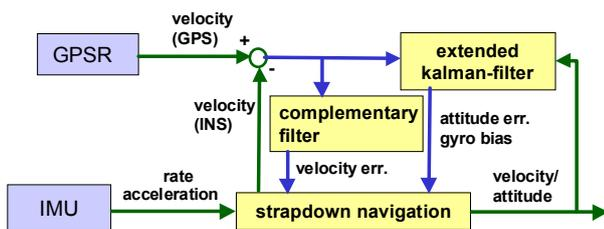
Figure 1. Block diagram of proposed GPS/INS
